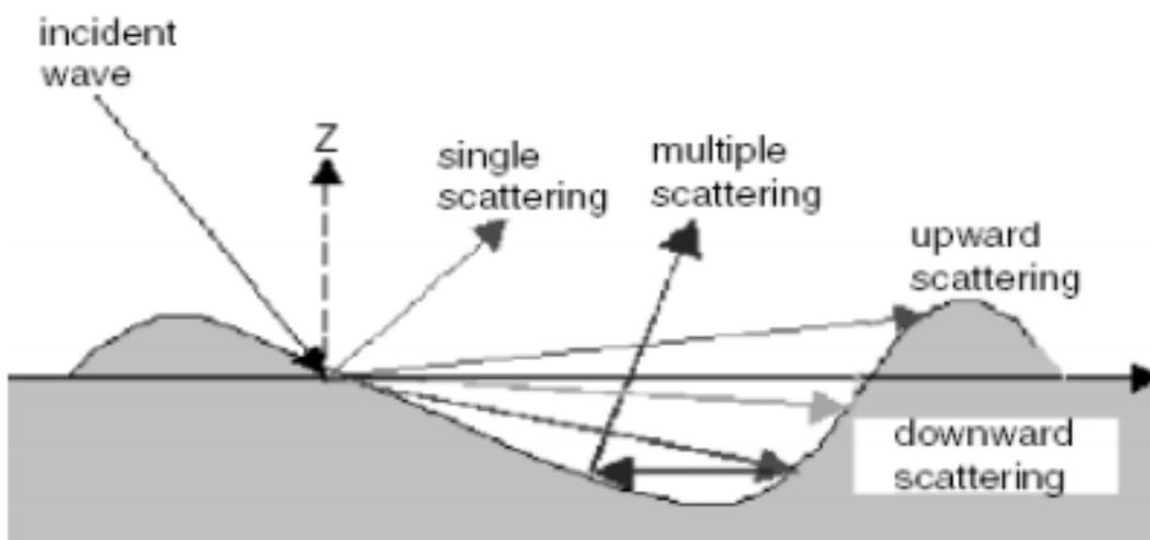
Fig. 3: Different type of surface scattering (Earth and planetary surfaces)
