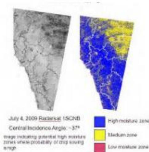
**Fig 6:** Typical relative soil moisture map produced using radarsat data
